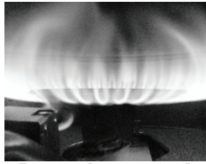
Proper burner and pilot burner pattern.
