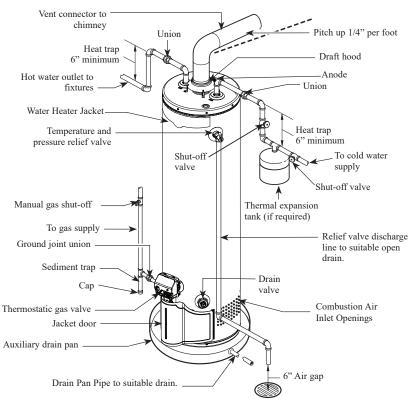
A new combination temperature and pressure relief valve, complying with the Standard for Relief Valves for Hot Water Supply Systems, ANSI Z21.22/CSA 4.4, is factory installed and must remain in the opening provided and marked for the purpose on the water heater. No valve of any type should be installed between the relief valve and the tank.
