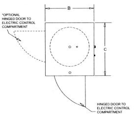
\*An oversized control panel may be required on models with inputs above 72 kW. An oversized control panel may increase the width and depth of the square jacket by up to 2\*.
