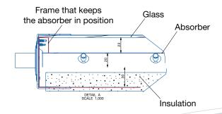
Collector with titanium selective absorber
