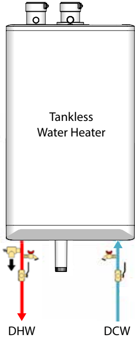
Figure 25: Overview of piping connections
