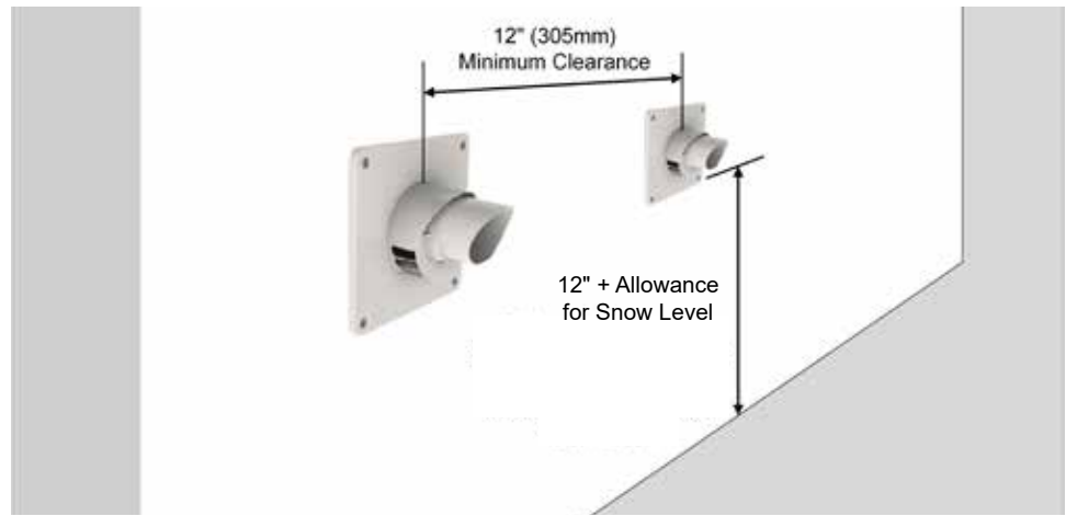
Figure 17: Horizontal Polypropylene Concentric Termination - Two Kits
