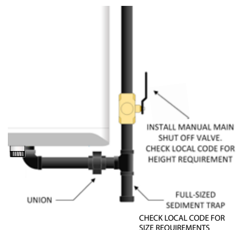
Figure 36: Gas Piping
