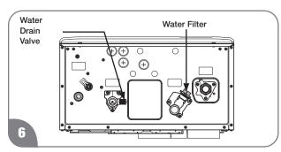
Find the water drain valve and the water filter located at bottom of the water heater.
