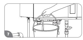
Using a suitable container to catch the water, remove the water drain valve from the base of the hot water outlet line, and the water filter from the base of the cold water inlet line.
