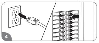
Turn on all electric power to the water heater. The remote control must be powered on prior to operating the water heater.
