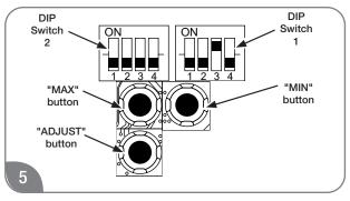
Within 30 seconds of turning the third switch ON, press the "Max button" or "Min button" on the control board to set the activation of this control.
