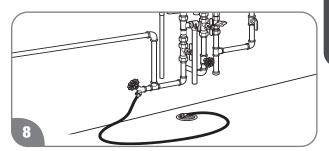
Connect a garden hose to the drain valve in the hot water outlet line and place the other end in a suitable drain. Open the drain valve until all the water has drained from the water heater. Leave water heater as is until placed back in service.
