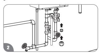
Install a ground joint union or ANSI design-certified semi-rigid or flexible gas appliance connector to the open end of the manual gas appliance shut-off valve. The NFGC, ANSI Z223.1 and CAN/CSA B149.1 codes mandate the use of manual gas shut-off valve.
