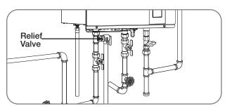
Annually check the operation of the pressure relief valve annually. Lifting the lever handle on the pressure-relief valve opens the valve to flush hot water through the discharge line to the drain. After several gallons have drained, release the lever handle to close the valve and stop draining.
