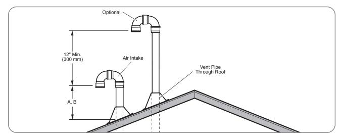
The following chart with diagrams details the minimum dimensional information needed to determine the proper location of the vertical vent terminal for direct-vent indoor tankless water heaters:
