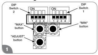
The factory setting for the switch should all be in the OFF position (Down).
