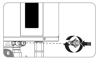
Replace the filter in the cold water inlet line and tighten until it is snug.
