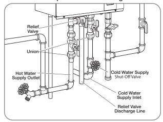
For safe operation of the water heater, be sure that:
