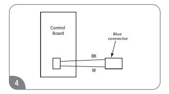
The wire harness for the recirculation pump is bundled with the wire harness from the control board. Find a blue connector with a black and a white wire.
