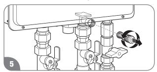
Close the shut-off valve and remove, clean, and replace the water filter.
