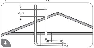
Determine the vent terminal height and install the vent pipe accordingly. Refer to "Vertical Vent Terminal Location" for clearance requirements.
