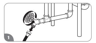
Disconnect drain hose. Make sure the drain valve is closed.
