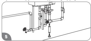
Install a sediment trap at the lowest portion of the gas line.
