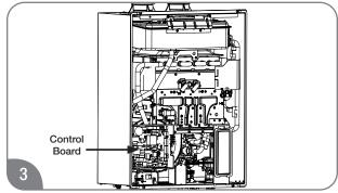
Find DIP Switch 1 and 2 located in the top-right portion of the control board.
