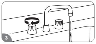
Open a hot water faucet slightly until the water stream is approximately 1/8 in. (0.3 cm). Be sure to check the flow periodically.
