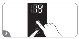
Press and hold the "▲"and "▼"button until "1Y" is displayed on the built-in display.
