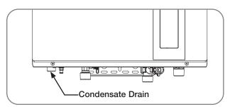
On a regular basis, inspect the condensate drain line to ensure the condensate is draining properly.
