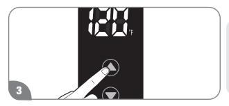
Press the UP adjustment button repeatedly until 120°F (49°C) shows in the LED display.
