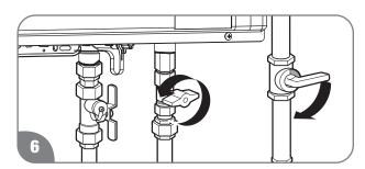
Open the gas shut-off valve(s).
