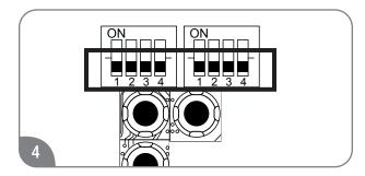
The factory settings for this switch should all be in the OFF position (DOWN), which is the A-0 setting.
