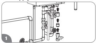
Install the manual gas appliance shut-off valve to the gas connection at the water heater.
