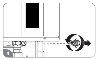
Unscrew the water filter from the base of the cold water inlet line and carefully slide it out of the line.
