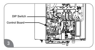
Find DIP Switch 1 located in the top-right portion at the control board. The switch labeled "DIP 1" is the right-most set of switches. If any DIP switches are on for venting/altitude settings, switch them to the OFF position.
