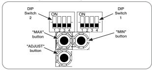
A-0 setting is default and factory setting. All dip switches are off.
