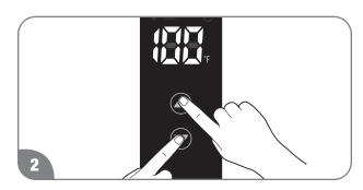
Press and hold DOWN button for 2 seconds. While holding the DOWN button, press the UP button. Release both buttons.
