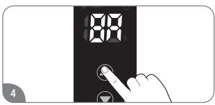
Press the "▲"or "▼"button until "8A" is displayed. Press and hold the power button on the build-in display for 1 second.
