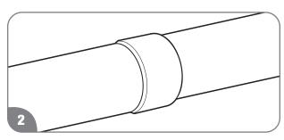
Attach the female end of the next vent pipe section to the male end of the 2-in./3-in. (5.1-cm/7.6-cm) vent pipe. See "Cementing Joints" on this Use and Care Manual.
