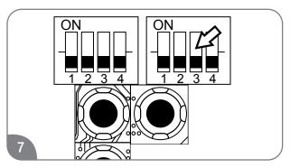
After setting the activation of this control, change the third switch on "DIP 1" to the OFF position (DOWN). Be sure to reapply any venting/altitude DIP switch settings.
