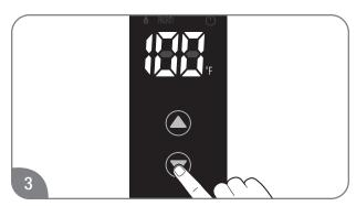
Press the DOWN adjustment button repeatedly until the lowest setting temperature shows in the LED display.
