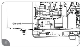
Connect the ground wire from the pump to a screw at the base of the water heater cabinet.
