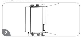
Remove the front cover panel on the water heater.
