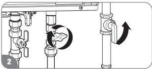
Close the gas shut-off valve(s).
