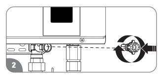
Reinstall the water filter in the base of the cold water inlet line, the water drain valve, and the water drain plug.
