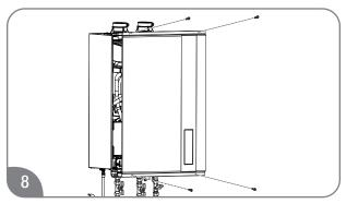
Replace the front cover panel and turn the remote ON. Turn the remote on before turning the water supply on.
