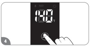
While "120" is shown on LED display, press and hold UP button for 5 seconds. "140" is shown on the LED display.
