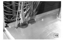
Wiring throughout the unit is neatly bundled and routed. Where wire harnesses go through the condenser bulkhead or blower deck, a molded wire harness assembly (19) provides an air-tight and water-tight seal, and provides strain relief. Care is also taken to tuck raw edges of insulation behind sheet metal to improve indoor air quality.
