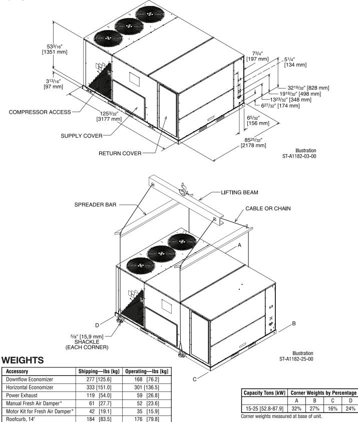
NOTES: \*Motorized Kit and Manual Fresh Air Damper must be combined for a complete Motorized Outside Air Damper Selection.
