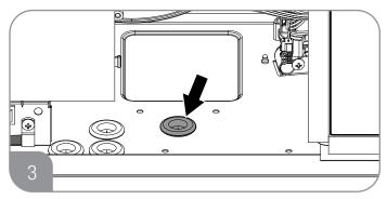
Locate junction box mounting location and power cord grommet.
