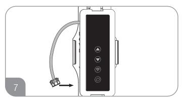
Have enough slack in wire to plug into the bottom of the display.
