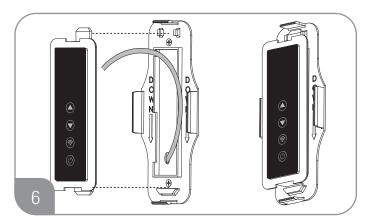
Rest display in "cup" at the bottom of mount and push into retention clips at the top.
