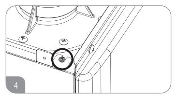
Tighten screws to secure the brackets to the unit.
