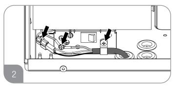
Remove power cable by disconnecting Molex connector, ground screw and strain relief.
