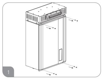
Remove 4 screws of Front Cover to access into unit.
