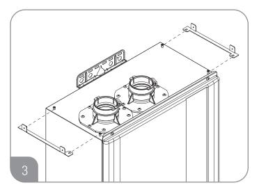
Slide mounting bracket onto screws. Before tightening, ensure bracket is inserted along guides fully.
