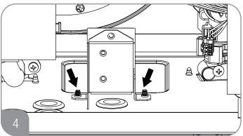
Mount Back of junction box with two screws provided.
