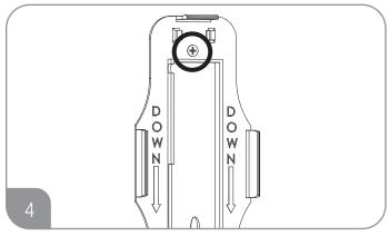
Ensure screw is flush to mount and does not protrude, as it will interfere with the display.
