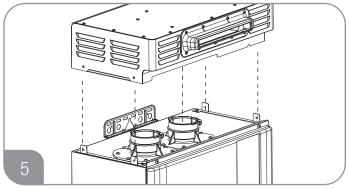
Place the exhaust hood on the top of the unit by aligning the exhaust pipe to the outlet flue connection of the unit.
