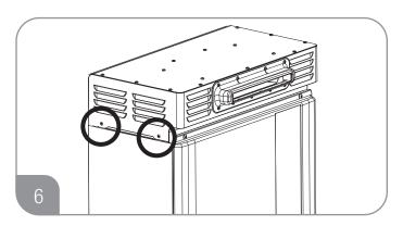
Secure the exhaust hood to the mounting brackets with 4 screws.
