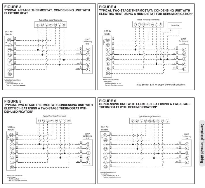
\*If maximum outlet temperature rise is desired, it is recommended that W1 and W2 be jumpered together.
