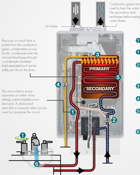
used to heat the water in the secondary heat exchanger before exiting the water heater.
