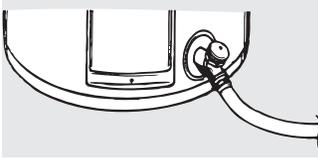
**▲CAUTION:** Shut off power to the water heater before draining water.
