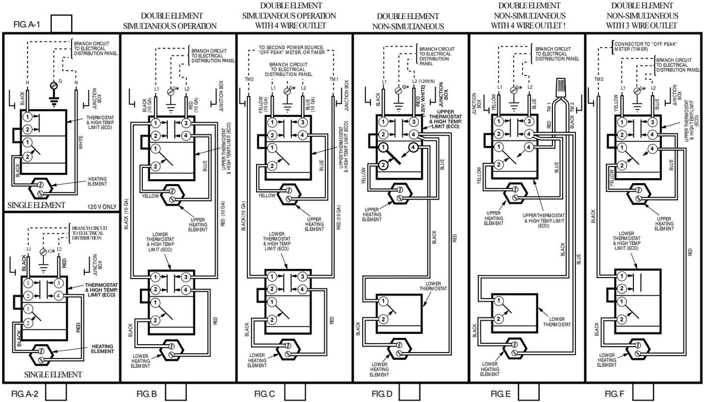
\* Grounding conductor may be required. Refer to Wiring Section of Manual
