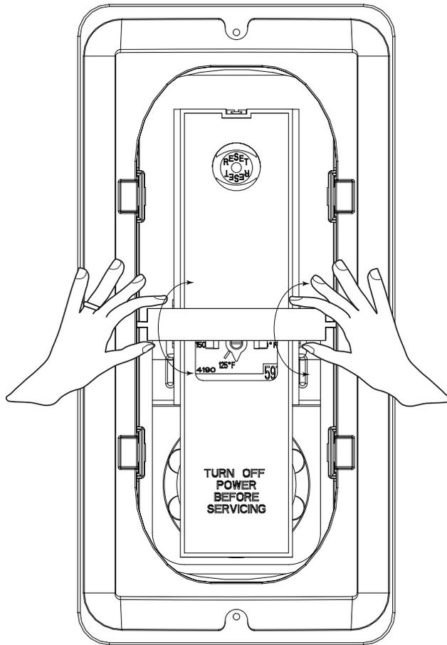
In order to replace the thermostat or heating element, remove the cavity insert crossbar by following the instructions below:
