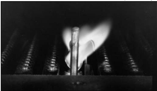
Figure 7. — Pilot Flame Pattern (Standard Burner)
