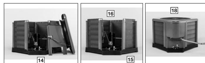
All units utilize strong formed louver panels which provide industry leading coil protection. Louver removal for coil cleaning is accomplished by removing one screw and lifting the panel out of the composite base pan. (17) All SA14 units utilize single row coils (16) making cleaning easy and complete, restoring the performance of the air conditioner back to out of the box performance levels year after year.
