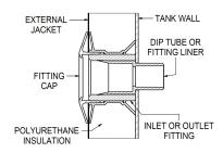
Diagram 4. Internal Water Pipework
