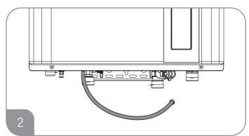
Run cable through wall to display location.
