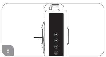
Ensure wire is tucked inside of the retention clip.
