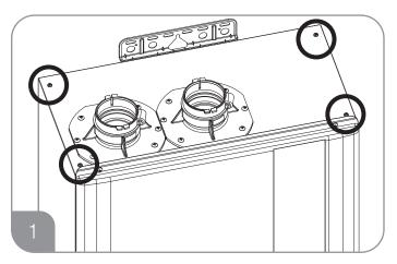
Locate 4 screws on top of the unit that will be used to mount the exhaust hood.
