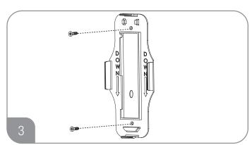
Use two screws to mount back of wall mount to wall/ desired location.
