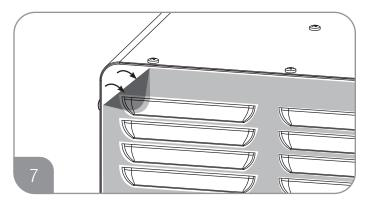
After completion of all installation steps, peel off protective film from all external surfaces.
