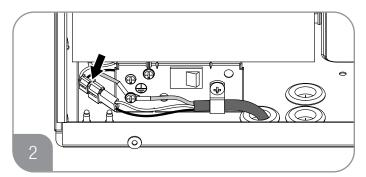
Remove power cable by disconnecting Molex connector.
