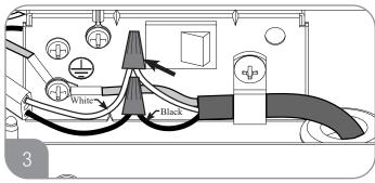
Connect wire harness to the power supply via wire nuts.
