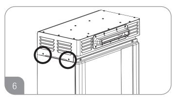
Secure the exhaust hood to the mounting brackets with 4 screws.
