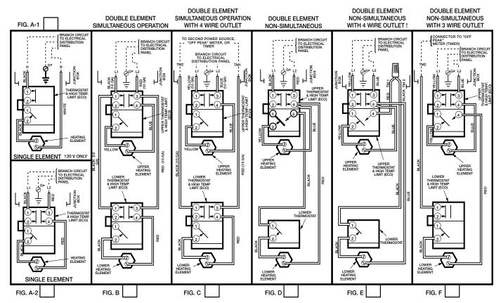
Grounding conductor may be required. Refer to Wiring Section of Manual
