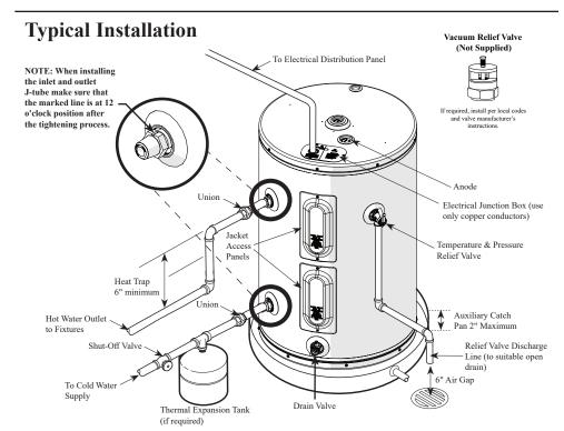
A new combination temperature and pressure relief valve, complying with the Standard for Relief Valves for Hot Water Supply Systems, ANSI Z21.22, is supplied and must be installed in the opening provided and marked for the purpose on the water heater. No valve of any type should be installed between the relief valve and the tank. Local codes shall govern the installation of relief valves.
