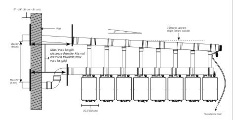
**NUMBER RUUD TRUNK OF UNITS PART NUMBER** DIAMETER SP20906A 2 SP20906B 6" 3 SP20906C 4 2 SP20908A SP20908B 3 SP20908C 4 SP20908D 8" 5 SP20908E 6 SP20908F 7 8 SP20908G SP20910A 2 SP20910B 3 SP20910C 4 5 SP20910D SP20910E 10" 6 SP20910F 7 SP20910G 8 SP20910H 9 SP20910J 10
