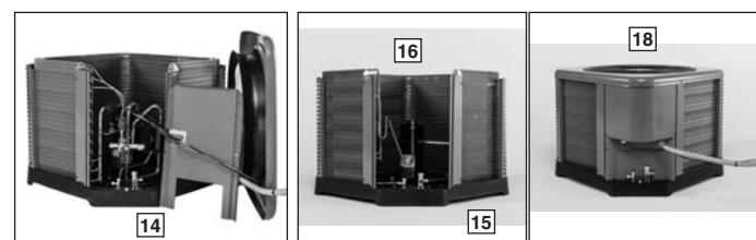
All units utilize strong formed louver panels which provide industry leading coil protection. Louver removal for coil cleaning is accomplished by removing one screw and lifting the panel out of the composite base pan (17). All RP16 units utilize single row coils (16) making cleaning easy and complete, restoring the performance of the heat pump back to out of the box performance levels year after year.
