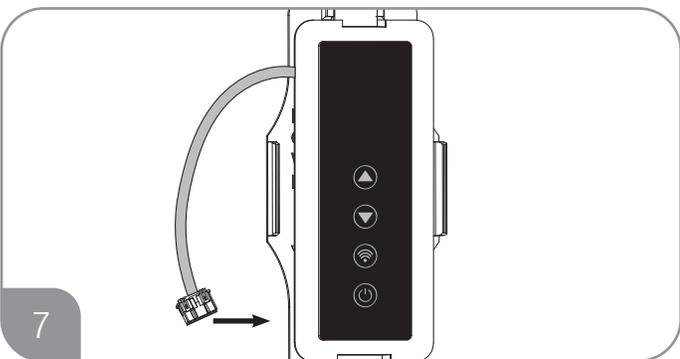
Have enough slack in wire to plug into the bottom of the display.
