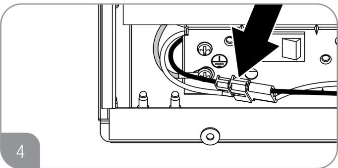
Reconnect the Molex connector of the wire harness to the unit.
