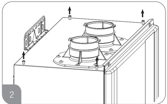
Loosen the four screws to prepare for the mounting brackets. (5 or 6 turns).
