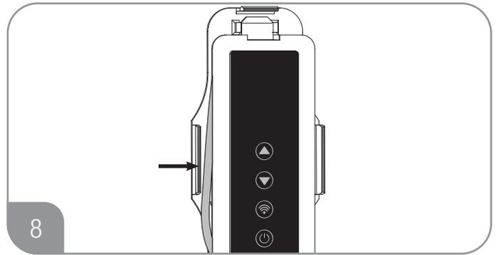
Ensure wire is tucked inside of the retention clip.
