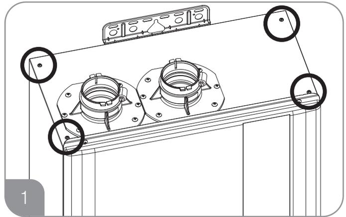
Locate 4 screws on top of the unit that will be used to mount the exhaust hood.
