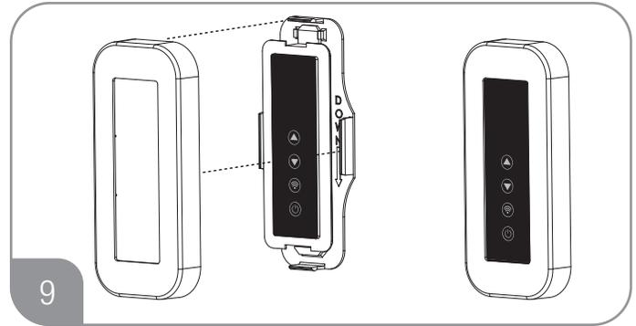
Front cover snaps onto the back of wall mount kit.
