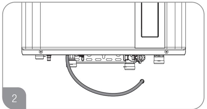
Run cable through wall to display location.
