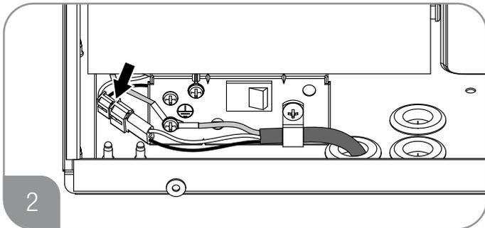
Remove power cable by disconnecting Molex connector.
