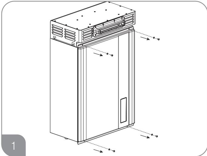
Remove 4 screws of Front Cover to access into unit.
