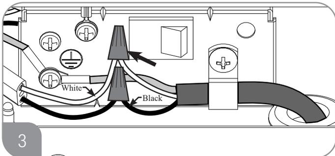
Connect wire harness to the power supply via wire nuts.
