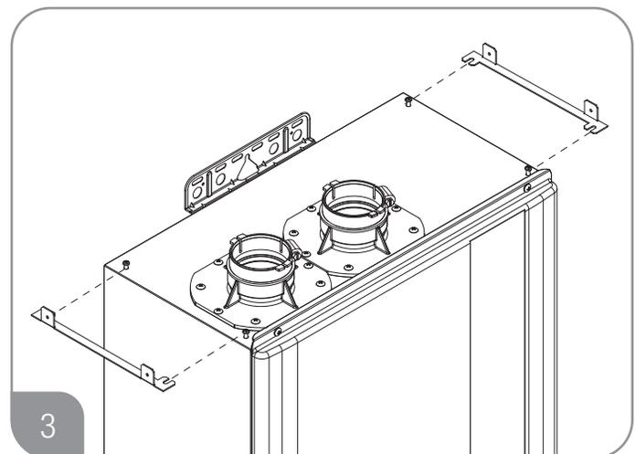
Slide mounting bracket onto screws. Before tightening, ensure bracket is inserted along guides fully.
