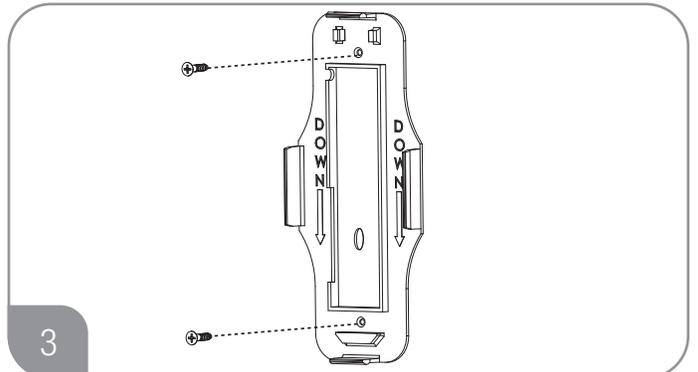
Use two screws to mount back of wall mount to wall/
