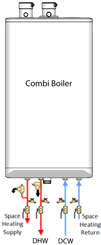
Figure 24: Overview of piping connections
