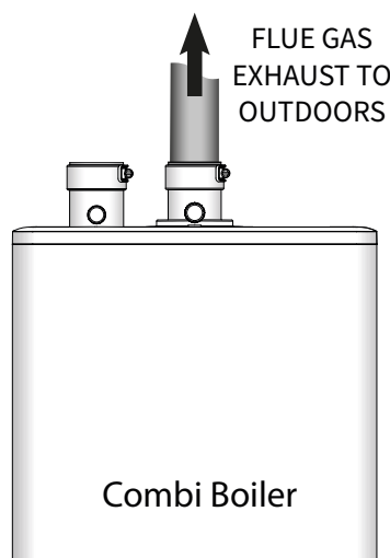
Figure 6: Basic exhaust vent assembly
