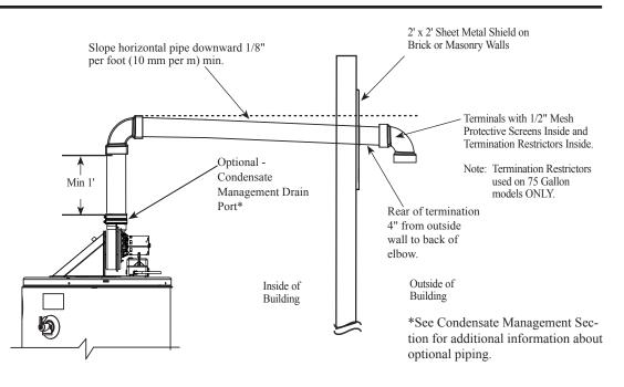
Horizontal Vent Terminal Installation
