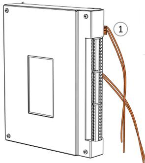
Figure 11 : Field wiring for (primary) pump –
