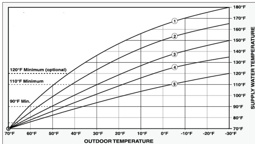
Figure 8 Characterized heating curve in advanced reset heating
