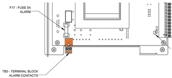
The alarm contacts will normally be open indicating that there is no alarm present. The contacts are closed when an alarm state is present and boiler operation has been disabled. This corresponds to when the boiler status bar on the display is red. The error that was detected creating the alarm state is recorded in the Error Log and displayed on the boiler status bar.
