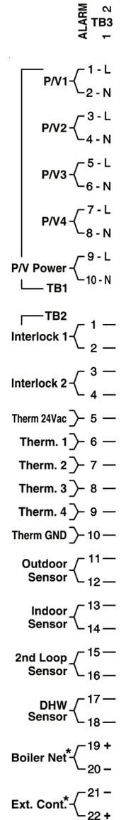
Figure 12 Controller's wiring strip
