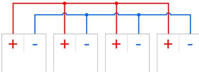
Figure 16 *Daisy-chain wiring*
