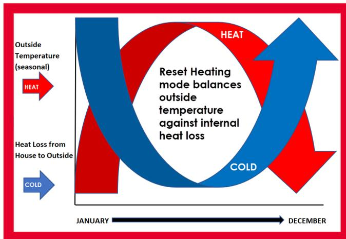
Figure 5 Heat loss vs outdoor temperature
