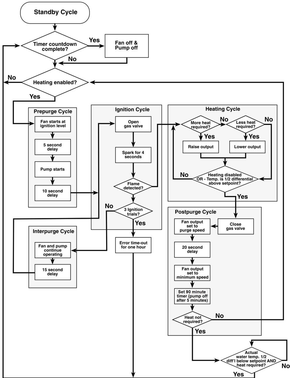
Figure 23 Sequence of Operation
