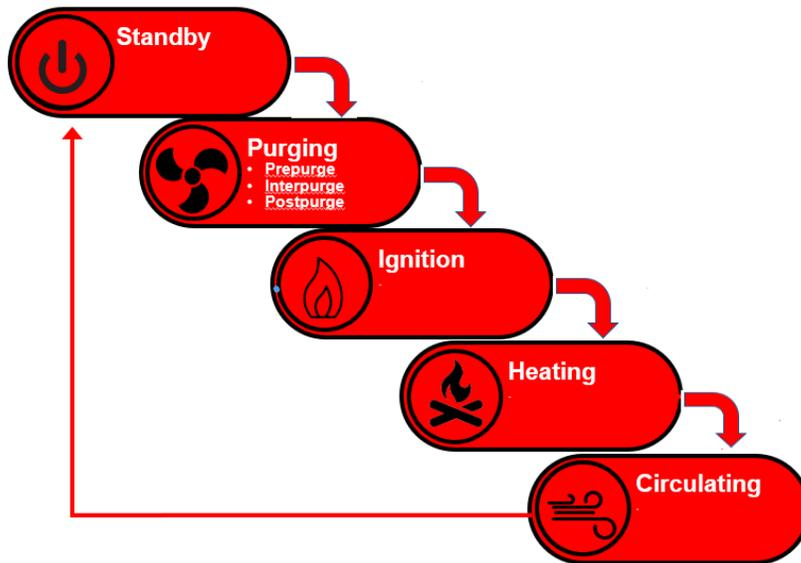
Figure 3 Stages of controller operation
