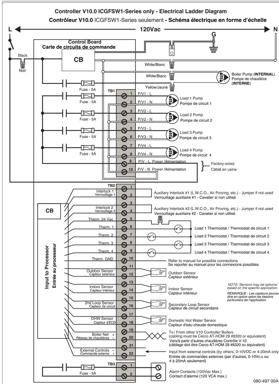
Figure 21 Combi Boiler - Controller diagram
