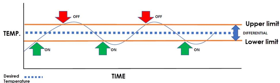
Figure 10 Boiler turns on/off according to differential high and low limits
