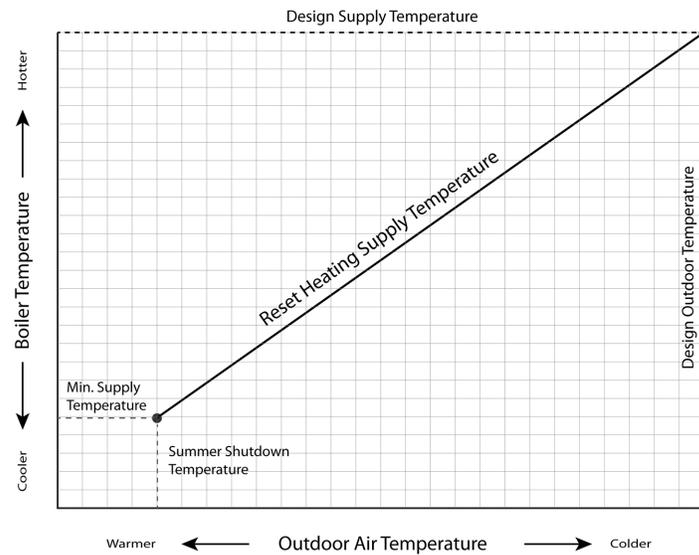
Figure 7 Standard "straight-line" reset heating
