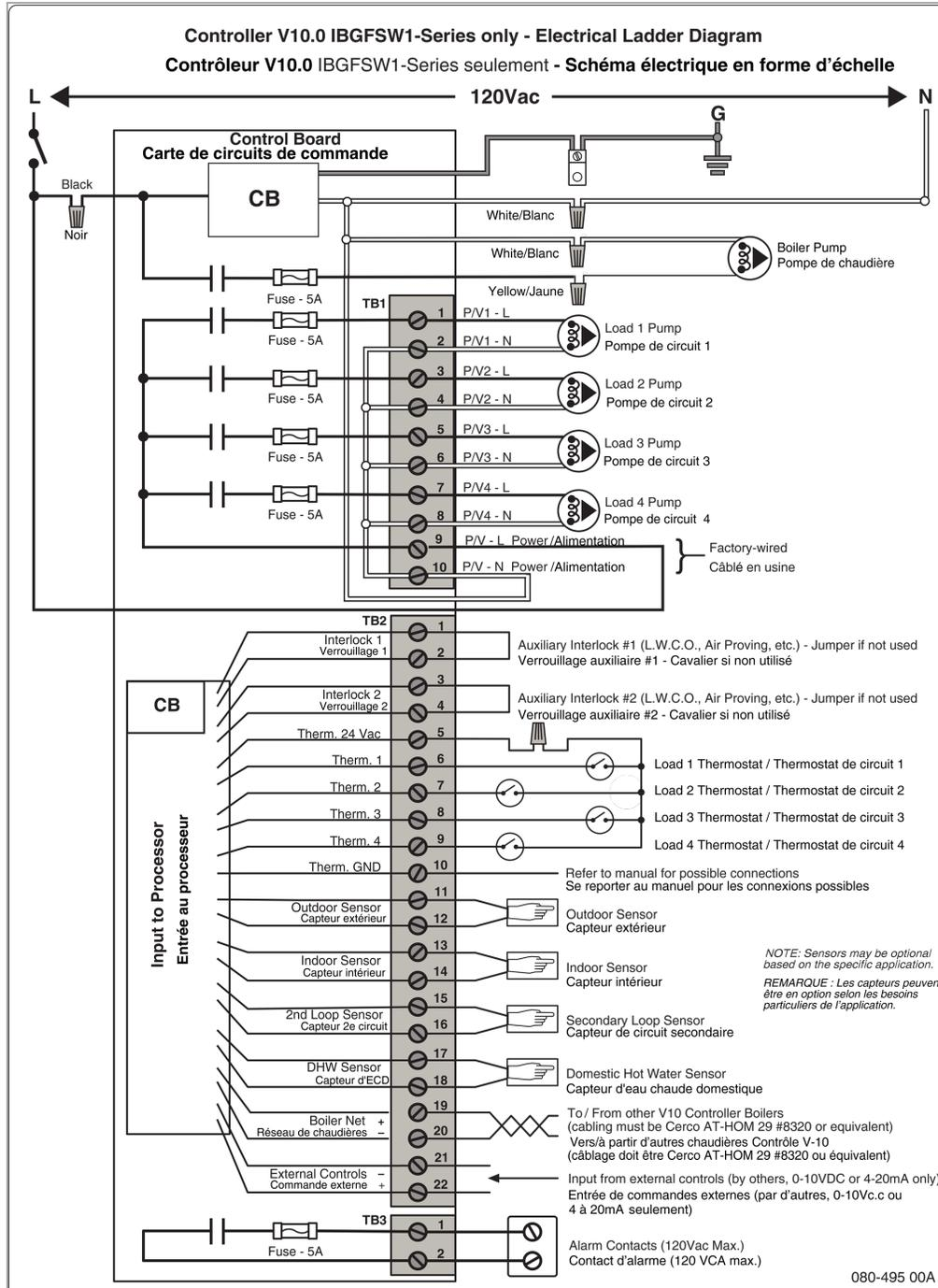
Figure 20 Boiler - Controller diagram
