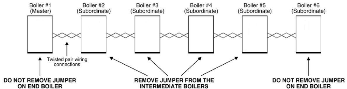
Figure 17 Circuit board jumper removal
