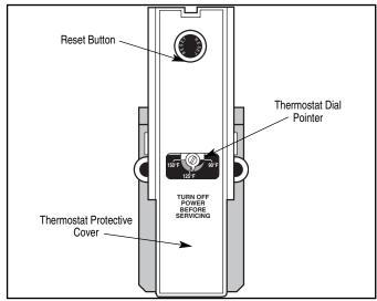
The illustration above shows the temperature adjustment dial used for setting the water temperature. Refer to Operation section of this manual for detailed instructions in how to adjust the thermostat(s).
