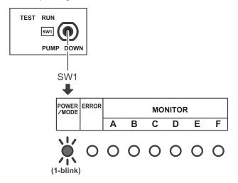
5. Press "TEST RUN" switch for more than 3 seconds.
