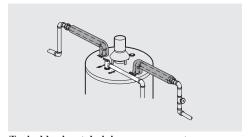
Typical horizontal piping arrangement
