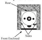
A WARNING: Combustible construction refers to adjacent walls and ceilings and should not be confused with combustible or flammable products and materials. Combustible and/or flammable products and materials should never be stored in the vicinity of this or any gas appliance.
