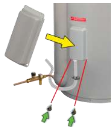
Step 30 refit electrical front cover
