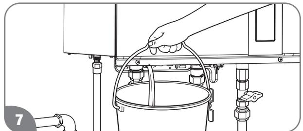
Using a suitable container to catch the water, remove the water drain valve from the base of the hot water outlet line, and the water filter from the base of the cold water inlet line.
