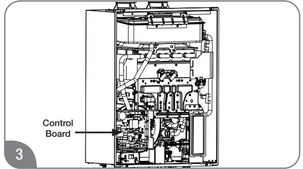
Find DIP Switch 1 and 2 located in the top-right portion of the control board.
