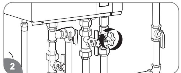
Turn the gas shut-off valve clockwise to the OFF position.
