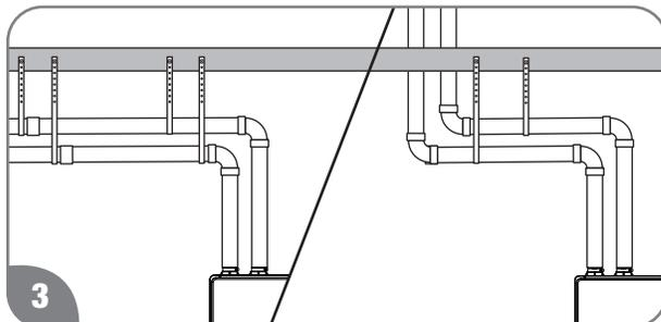
Support vertical and horizontal runs as described on page 23. Vertical supports are required every 4 ft. (1.2 m) along a vertical pipe route, after every transition to vertical, and after every offset elbow.
