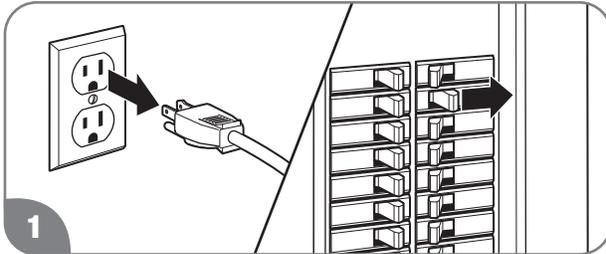
Disconnect all electric power to the water heater.
