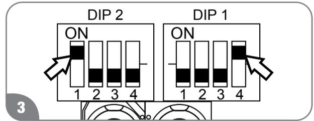
To select Energy Saver mode, change the fourth switch on "DIP switch 1" to the ON position (UP).
