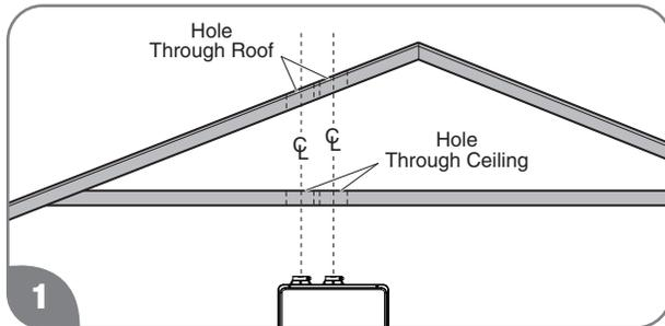
Cut a hole through the roof and interior ceiling to accommodate the vent pipes.
