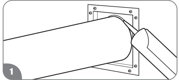
1 Apply silicone sealant or silicone/latex caulk to seal the vent pipe to the vent coupling to permit field disassembly for annual inspection and cleaning. Completely seal where it passes through the wall plate and where it is attached to the structure.
