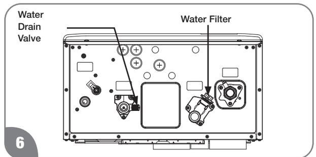
Find the water drain valve and the water filter located at bottom of the water heater.
