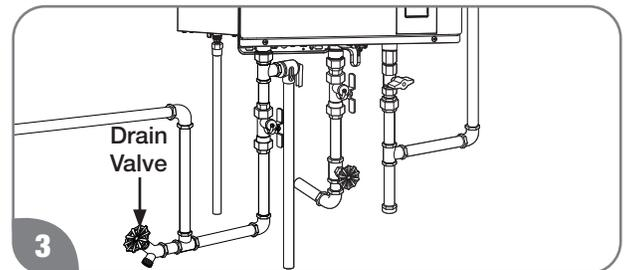
Drain the water heater. See "Draining the Water Heater" section.
