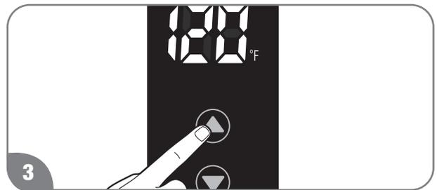
3 Press the UP adjustment button repeatedly until 120°F (49°C) shows in the LED display.
