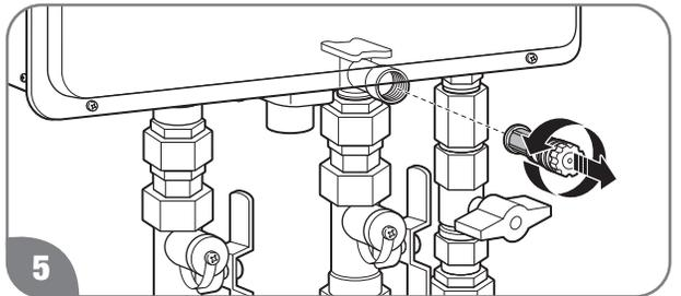
Close the shut-off valve and remove, clean, and replace the water filter.
