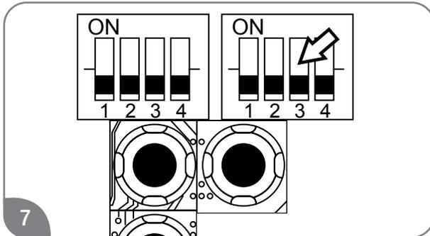
After setting the activation of this control, change the third switch on “DIP 1” to the OFF position (DOWN). Be sure to reapply any venting/altitude DIP switch settings.
