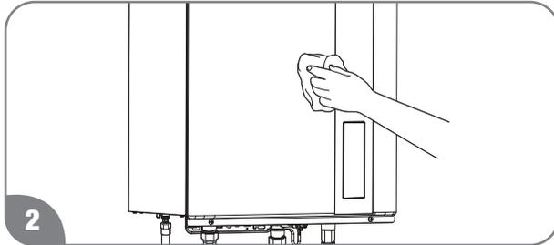
Clean the water heater with a damp soft cloth and mild detergent. Gently wipe and completely dry all surfaces.
