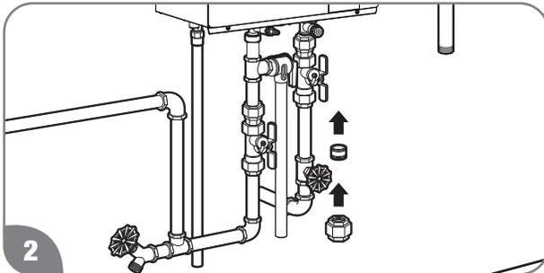
2 Install a ground joint union or ANSI design-certified semi-rigid or flexible gas appliance connector to the open end of the manual gas appliance shut-off valve. The NFGC, ANSI Z223.1 and CAN/CSA B149.1 codes mandate the use of manual gas shut-off valve.
