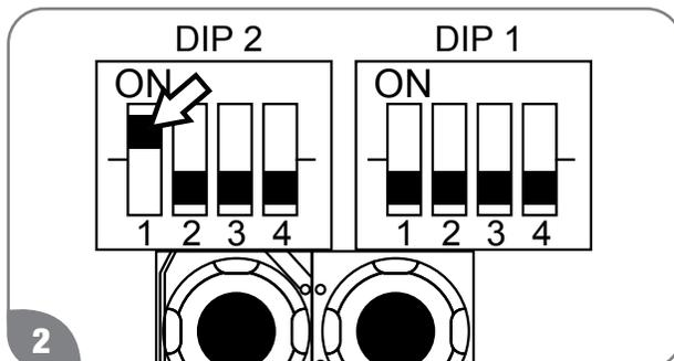
Change the first switch on "DIP switch 2" to the ON position (UP). Performance mode is selected.
