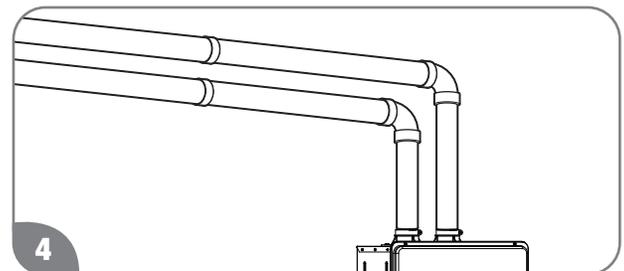
4 Complete the rest of the vent pipe installation to the water heater's flue outlet and air intake.
