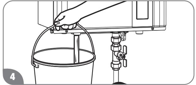
Open the shut-off valve in the COLD water Inlet line to check the water flow through the water heater.
