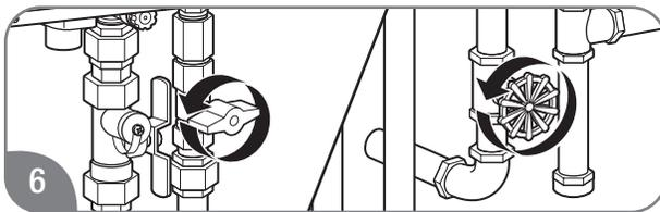
Turn on the gas and water to the water heater by opening the shut-off valves.
