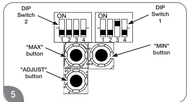
Within 30 seconds of turning the third switch ON, press the "Max button" or "Min button" on the control board to set the activation of this control.
