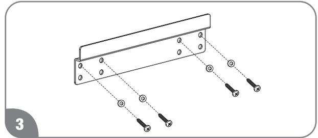
Attach the mounting bracket to the wall and secure it by 4 screws and washers. Make sure it is level and that it can support the weight of the water heater.
