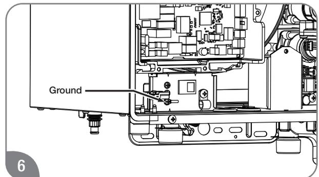
6 Connect the ground wire from the pump to a screw at the base of the water heater cabinet.
