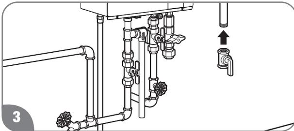
3 Install a manual gas supply line shut-off valve to the end of the gas supply line.
