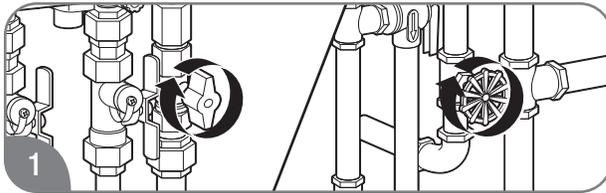
Turn off the gas and water to the water heater by closing the shut-off valves.
