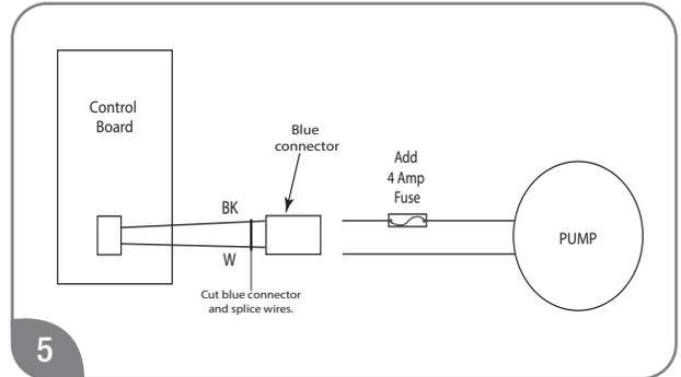
5 To connect to the pump, cut the blue connector, splice the wires, and add a 4 amp fuse to the hot wire of the pump. Rheem recirculation pump kit includes a molex connector and a 4 amp fuse so splicing wires is not required.
