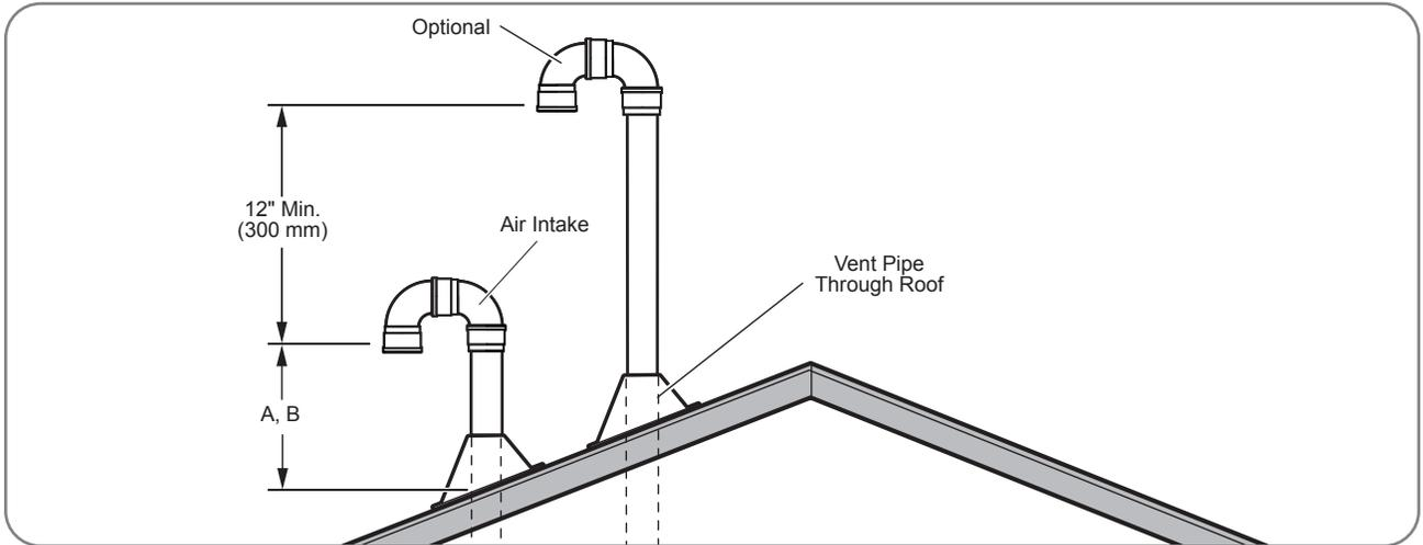
The following chart with diagrams details the minimum dimensional information needed to determine the proper location of the vertical vent terminal for direct-vent indoor tankless water heaters:
