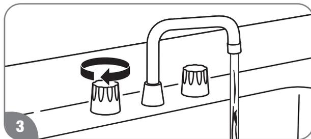
Open a hot water faucet slightly until the water stream is approximately 1/8 in. (0.3 cm). Be sure to check the flow periodically.
