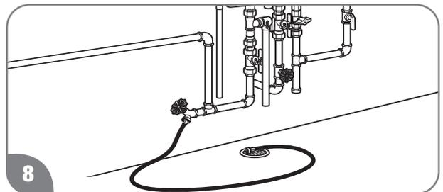
Connect a garden hose to the drain valve in the hot water outlet line and place the other end in a suitable drain. Open the drain valve until all the water has drained from the water heater. Leave water heater as is until placed back in service.
