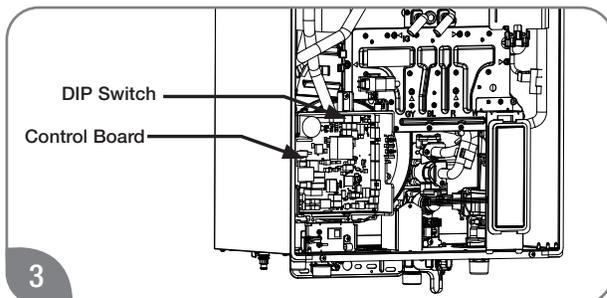
Find DIP Switch 1 located in the top-right portion at the control board. The switch labeled “DIP 1” is the right-most set of switches. If any DIP switches are on for venting/altitude settings, switch them to the OFF position.
