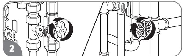
2 Turn off the gas and water to the water heater by closing the shut-off valves.
