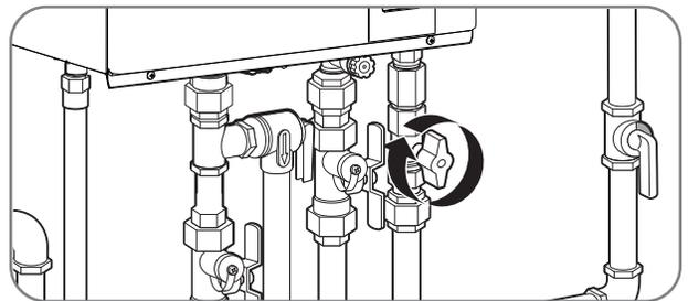
The water heater and its manual gas shut-off valve must be disconnected from the gas supply piping system during any pressure testing of the system at test pressures in excess of 1/2 psi (3.5 kPa).
