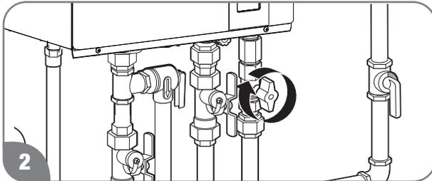
Turn the gas shut-off valve clockwise to the OFF position. This valve is located on the outside of the water heater. Wait 5 minutes to clear any gas. If you don't smell gas, proceed to Step 3.
