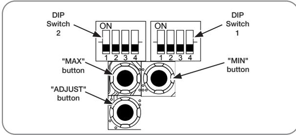
A-0 setting is default and factory setting. All dip switches are off.
