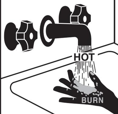
Water temperature over 125°F (52°C) can cause severe burns instantly or death from scalds.
