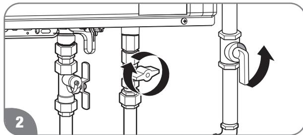
Close the gas shut-off valve(s).
