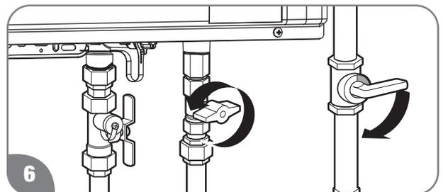
6 Open the gas shut-off valve(s).
