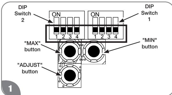
The factory setting for the switch should all be in the OFF position (Down).
