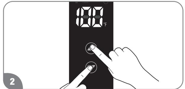
2 Press and hold DOWN button for 2 seconds. While holding the DOWN button, press the UP button. Release both buttons.
