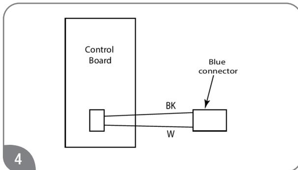
4 The wire harness for the recirculation pump is bundled with the wire harness from the control board. Find a blue connector with a black and a white wire.
