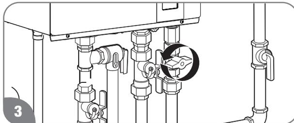
Turn the gas shut-off valve counterclockwise to the ON position.
