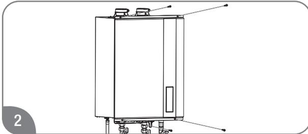
Remove the front cover panel on the water heater.
