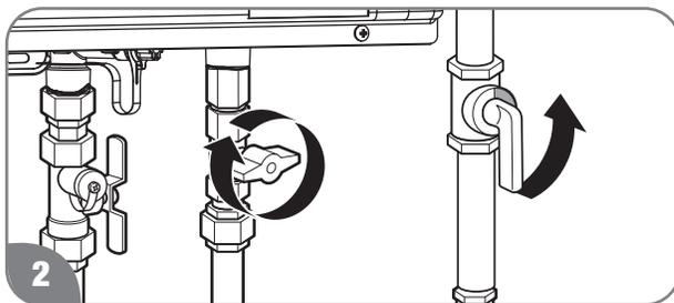
Close the gas shut-off valve(s).
