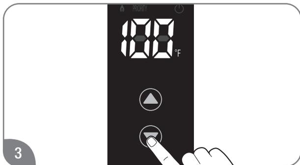
3 Press the DOWN adjustment button repeatedly until the lowest setting temperature shows in the LED display.
