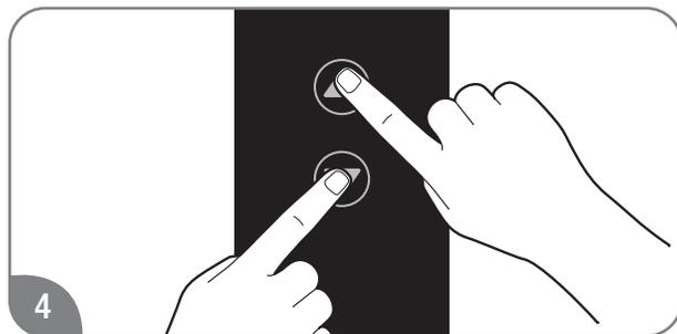
4 Press and hold the DOWN and UP adjustment button for 5 to 10 seconds.
