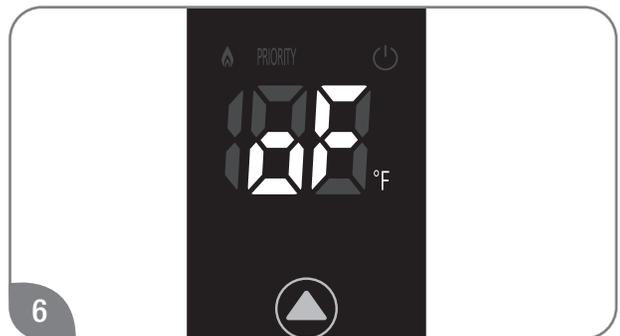
LED display on the built-in control shows “oF”.
