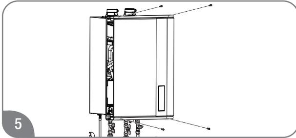
Replace the front cover panel on the water heater.
