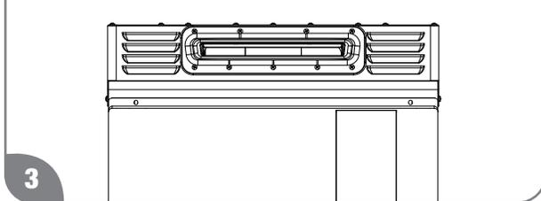
Check the air intake and vent outlet for blockage and/or debris.
