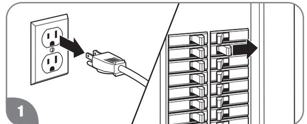
Disconnect all electric power to the water heater.
