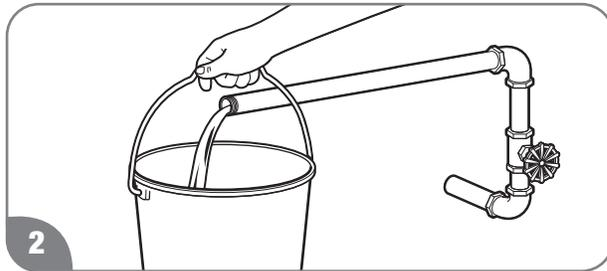
Before attaching the water line to the water heater, open the shut-off valve. Run the water until it has purged all contaminants (sand, debris, air, caulking, etc.).
