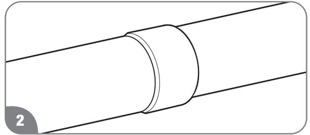
2 Attach the female end of the next vent pipe section to the male end of the 2-in./3-in. (5.1-cm/7.6-cm) vent pipe. See "Cementing Joints" on this Use and Care Manual.
