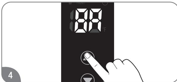
Press the “▲” or “▼” button until “8A” is displayed. Press and hold the power button on the built-in display for 1 second.
