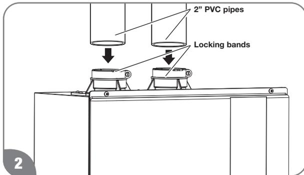
Insert a 2" PVC pipes slowly into an air intake connector and a flue connector located on top of the water heater until they stop. Tighten 2 locking bands to secure 2" PVC pipes.
