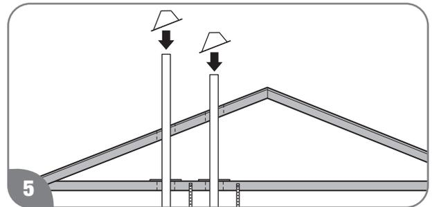
Install adequate flashing where the vent pipe passes through the roof.
