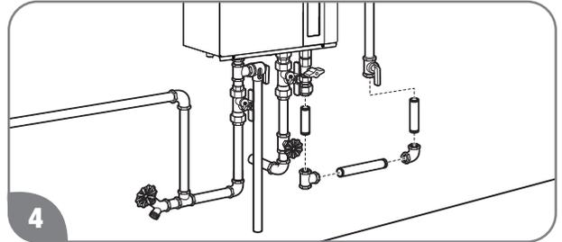
4 Using the proper-size piping, fittings, and components, build the gas supply line to the water heater.
