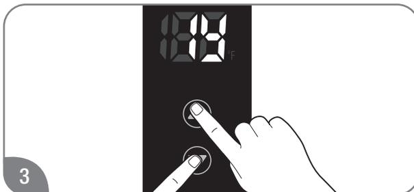
Press and hold the “▲” and “▼” button until “1Y” is displayed on the built-in display.
