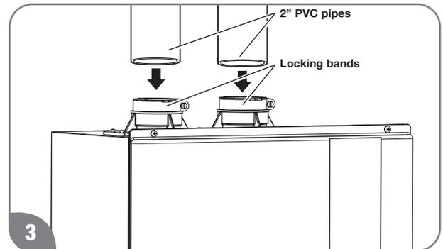
3 Insert a 2" PVC pipes slowly into an air intake connector and a flue connector located on top of the water heater until they stop. **DO NOT** use cement. Tighten 2 locking bands to secure 2" PVC pipes.
