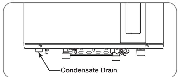
On a regular basis, inspect the condensate drain line to ensure the condensate is draining properly.
