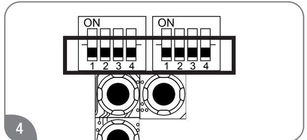
The factory settings for this switch should all be in the OFF position (DOWN), which is the A-0 setting.
