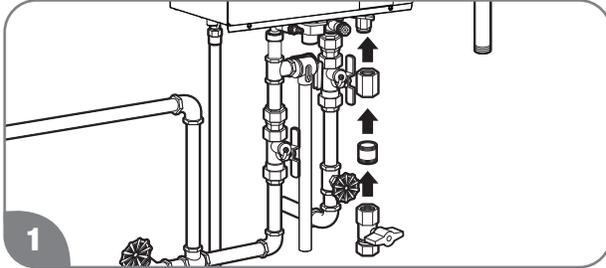
1 Install the manual gas appliance shut-off valve to the gas connection at the water heater.
