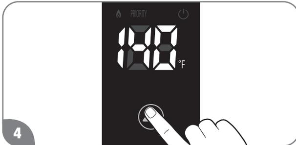
4 While "120" is shown on LED display, press and hold UP button for 5 seconds. "140" is shown on the LED display.
