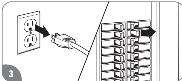
At least 10 seconds after Step 1, unplug the water heater or disconnect the power supply at the circuit breaker box.
