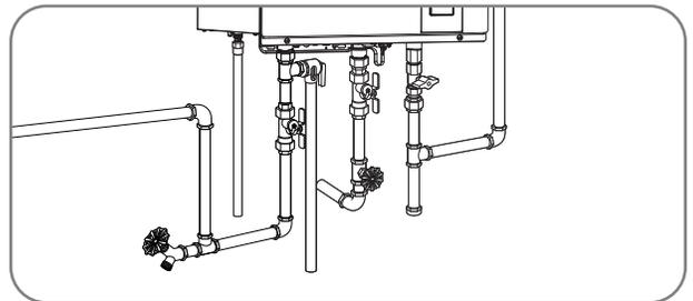
It is recommended to use unions and flexible copper connections at the COLD and HOT water lines. They allow the water heater to be disconnected easily for servicing.
