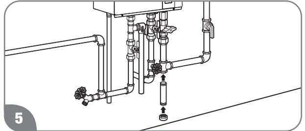
5 Install a sediment trap at the lowest portion of the gas line.
