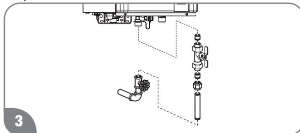
Install a service valve on the end of the COLD water supply line and connect it to the water inlet on the water heater.
