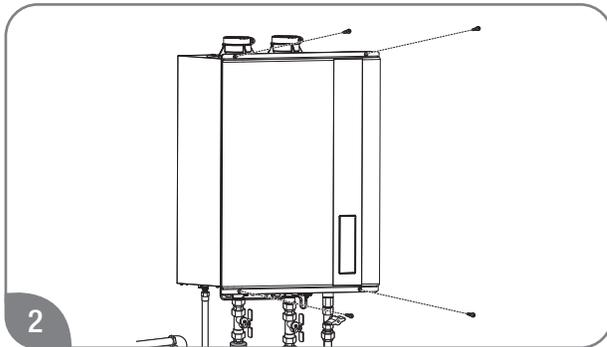
Remove the front cover panel on the water heater and ensure the remote is OFF.
