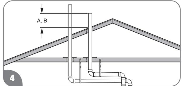
Determine the vent terminal height and install the vent pipe accordingly. Refer to "Vertical Vent Terminal Location" for clearance requirements.
