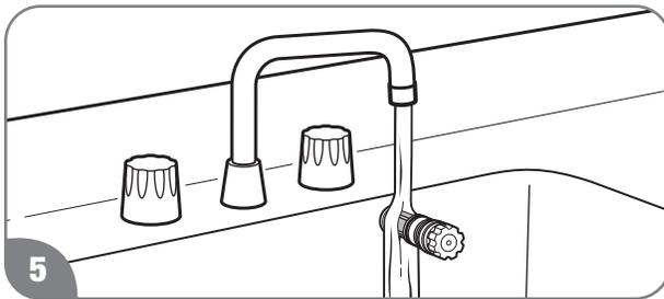
Clean the water filter under running water. To remove severe sediment and dirt, use a soft brush.
