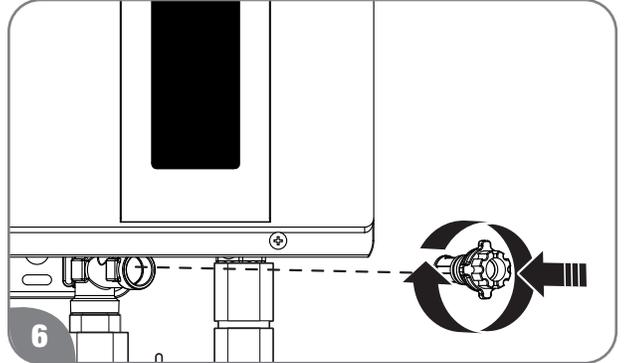
Replace the filter in the cold water inlet line and tighten until it is snug.
