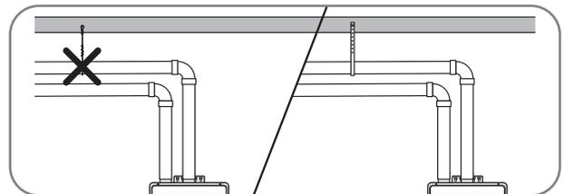
The unit may be vented horizontally through a wall or vertically through the roof. Pipe runs must be adequately supported along both vertical and horizontal runs.
