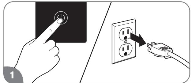
Turn off the water heater and disconnect the electrical power supply.
