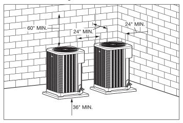
The outdoor unit must not be connected to any duct work. Do not locate unit under a roof drip; if necessary, install gutters, etc., to prevent water run-off from hitting the unit. To prevent air recirculation, it is recommended that the unit not be installed under an overhang, but if necessary **allow a minimum of 60 inches [1524 mm] above the unit for air discharge.**
