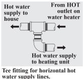
Tee fitting must be installed as shown. This ensures that any air in the water lines will be
