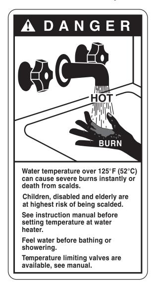
NOTICE: Mixing valves are recommended for reducing point of use water temperature by mixing hot and cold water in branch water lines. It is recommended that a mixing valve complying with the Standard for Temperature Actuated Mixing Valves for Hot Water Distribution Systems, ASSE 1017 be installed. See pages 18 & 19 for more details and contact a licensed plumber or the local plumbing authority for further information.
