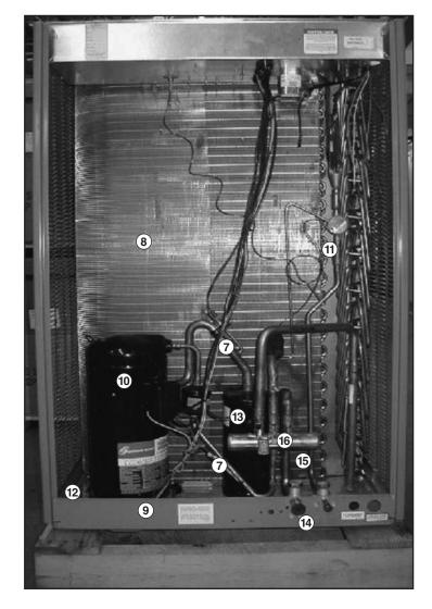
8. COIL—Constructed with copper tubes and aluminum fins mechanically bonded to tubes for maximum heat transfer capabilities. All coil assemblies are leak tested up to 550 PSIG (3792 kPa) internal pressure.
