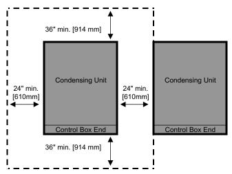
The unit must not be connected to any duct work. Do not locate unit under a roof drip; if necessary, install gutters, etc., to prevent water run-off from hitting the unit. To prevent air recirculation, it is recommended that the unit not be installed under an overhang, but if necessary **allow a minimum of 60 inches** [1524 mm] above the unit for air discharge.
