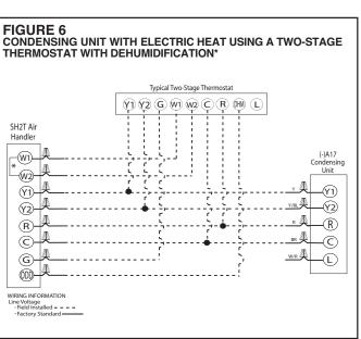
\*If maximum outlet temperature rise is desired, it is recommended that W1 and W2 be jumpered together.
