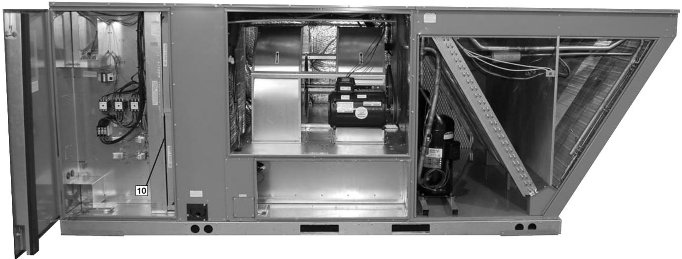
Inside the control box (11), each electrical component is clearly identified with a label that matches the component to the wire diagram for ease of trouble shooting. All wiring is numbered on each end of the termination and color-coded to match the wiring diagram. The control transformer has a low voltage circuit breaker that trips if a low voltage electrical short occurs. There is a blower contactor and contactor for each compressor.
