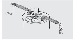
Typical horizontal piping arrangement
