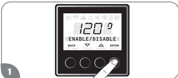
1 Press the "MODE" button. After the LCD displays "ENABLE/DISABLE", press the "ENTER" button.
