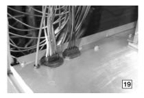
Wiring throughout the unit is neatly bundled and routed. Where wire harnesses go through the condenser bulkhead or blower deck, a molded wire harness assembly (19) provides an air-tight and water-tight seal, and provides strain relief. Care is also taken to tuck raw edges of insulation behind sheet metal to improve indoor air quality.
