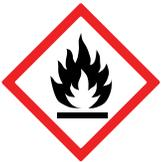
This symbol indicates that this appliance uses a flammable refrigerant. If the refrigerant is leaked and is exposed to an external ignition source, there is a risk of fire.
