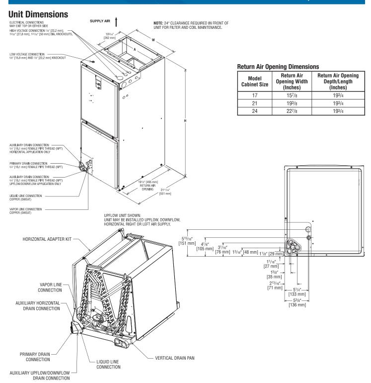
UPFLOW UNIT SHOWN: UNIT MAY BE INSTALLED UPFLOW, DOWNFLOW, HORIZONTAL RIGHT OR LEFT AIR SUPPLY.
